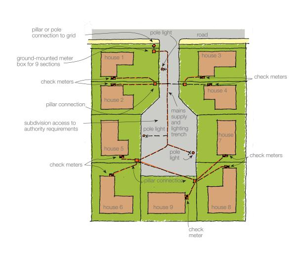
Schematic layout of a common power supply © BRANZ 2010
