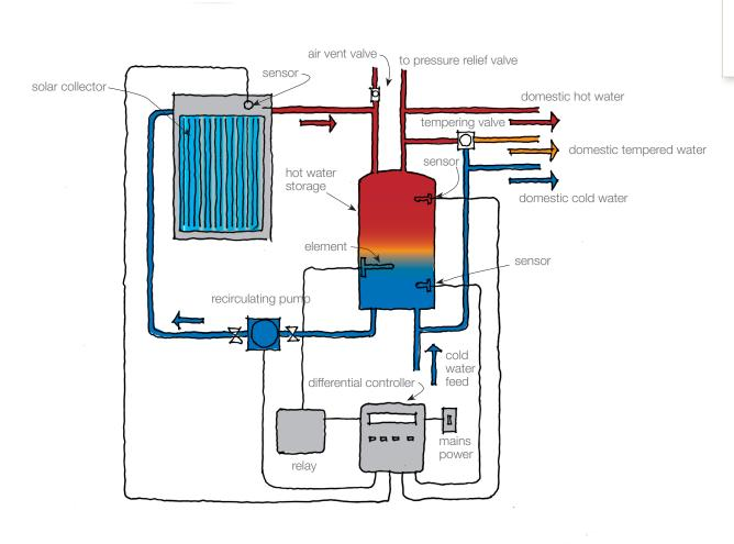
Schematic of wiring and controls for solar water heating © BRANZ 2010
