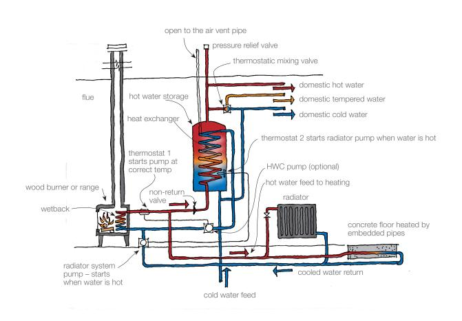
Schematic wiring diagram for wetback water and space heating © BRANZ 2010
