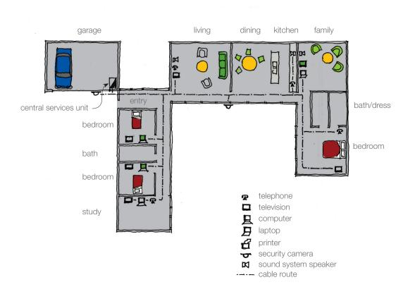
Schematic drawing of cable layout for home network system © BRANZ 2010
