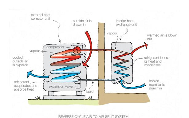
Heat pump Schematic diagram of how a heat pump operates in heating mode.
