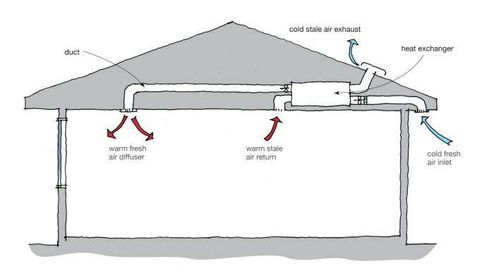
Schematic of typical heat recovery ventilation system.
