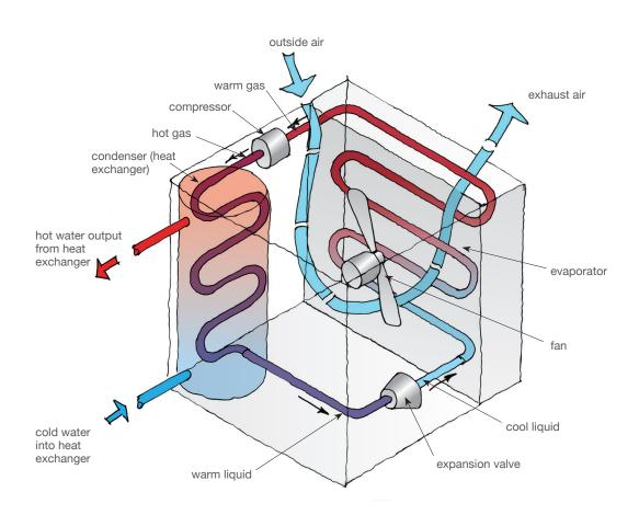
Heat pump water heater cycle.
