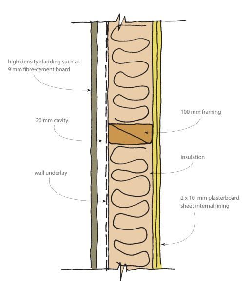
External sound envelope (fibre-cement cladding)
