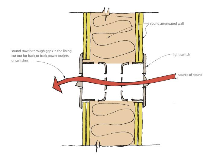
Sound paths through electrical fittings Sound will travel through any break in an acoustic system such as back-to-back power outlets. This will reduce the effectiveness of the acoustic system.
