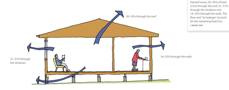
6–9% through the air leakage
