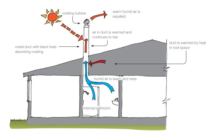
Principle of a solar chimney.
