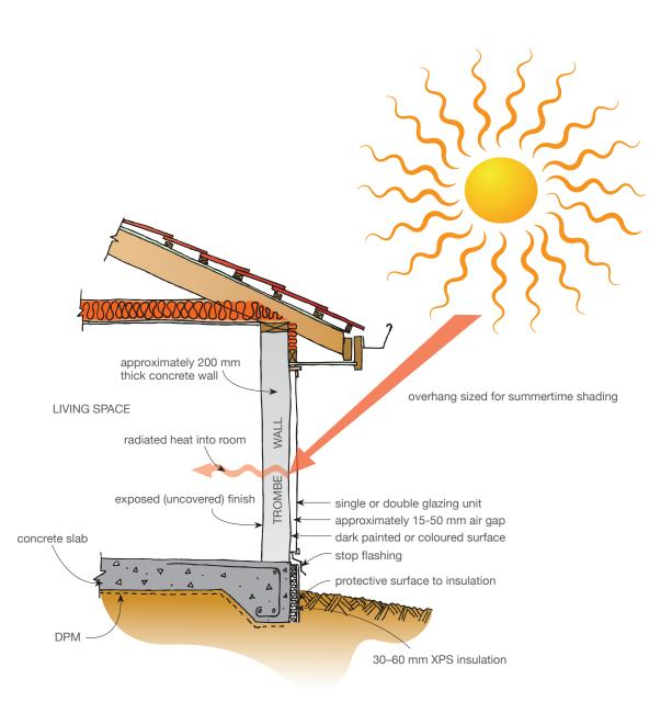
Basic principle of Trombe wall construction
