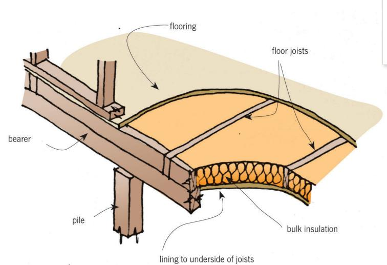
Suspended timber floor with bulk insulation and lining
