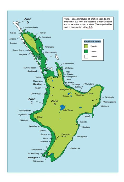
© Copyright Standards New Zealand 2012. Figure 4.2 Exposure zones from NZS 3604:2011 has been reproduced with permission from Standards New Zealand under Copyright Licence 000988.
