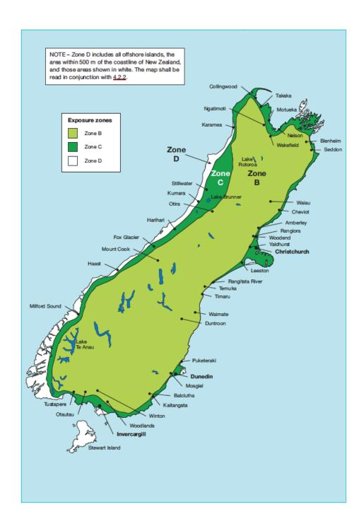
$^{\circ}$  Copyright Standards New Zealand 2012. Figure 4.2 Exposure zones from NZS 3604:2011 has been reproduced with permission from Standards New Zealand under Copyright Licence 000988.
