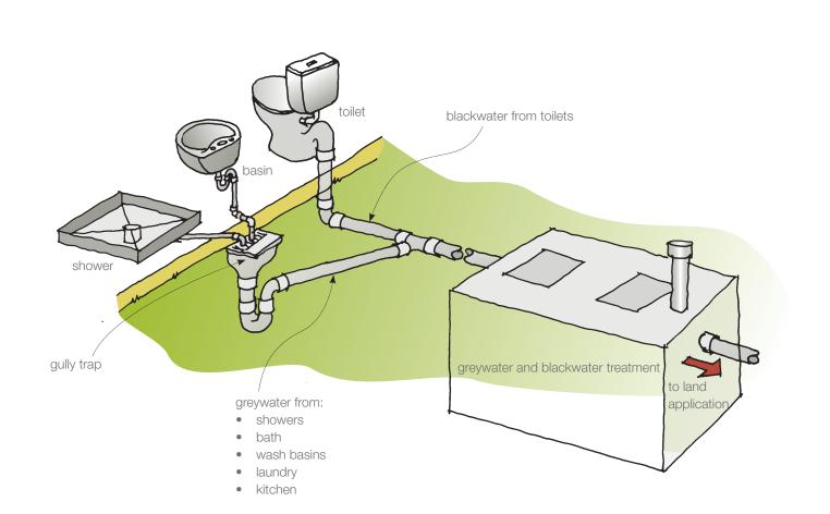
Schematic of on-site domestic wastewater treatment Where a sewerage
