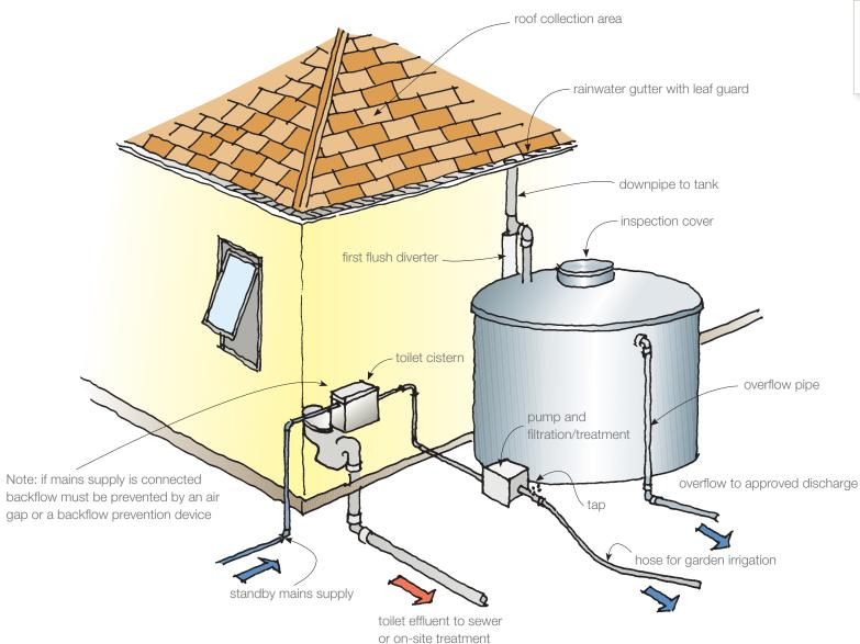
Schematic drawing of rainwater storage system for irrigation and toilet flushing
