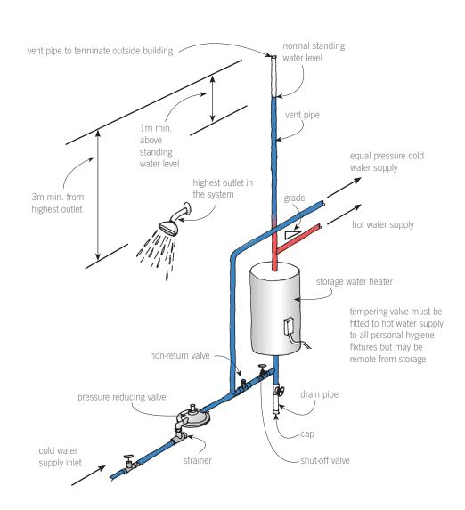
Low pressure, open-vented pressure-reducing valve storage water heater system
