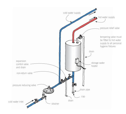
Low pressure, unvented pressure-reducing valve storage water heater system © BRANZ 2009
