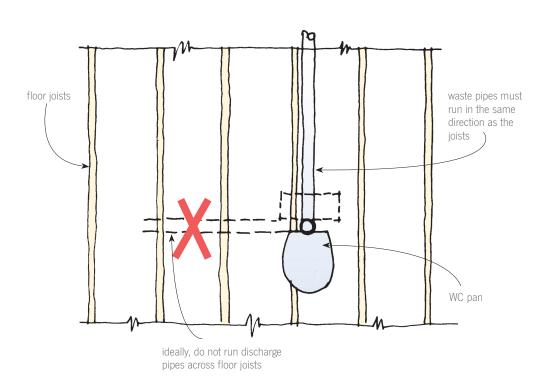
Discharge pipes within floor depth © BRANZ 2009
