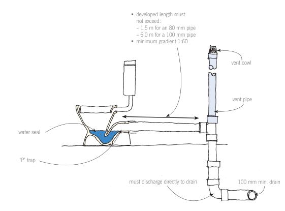
'P' trap soil fixture connected to drain and using the drain vent as a fixture vent
